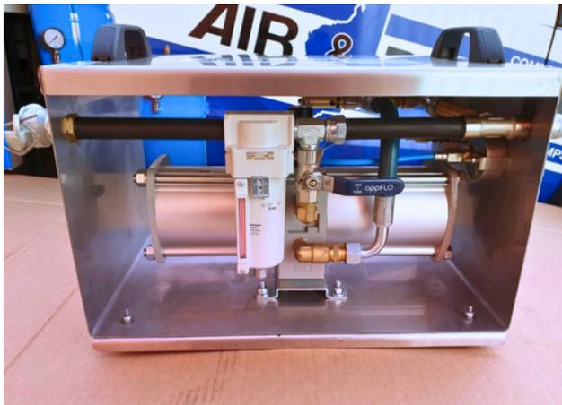
Tailored air multiplier designed for a client in the tyre industry. This innovation enables the client to double the pressure generated by their air compressor, enhancing tire inflation efficiency. Designed and manufactured in our Belmont workshop
