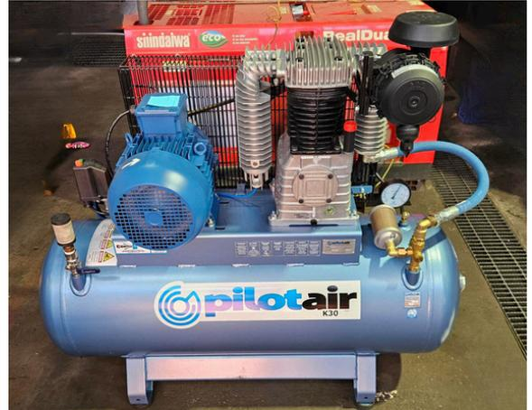
New PilotAir K30 was modified to include continuous running, allowing the compressor to run continuously without the need to start and stop. This reduces the strain on the generator greatly while in use. **Arc Infrastructure, WA**
