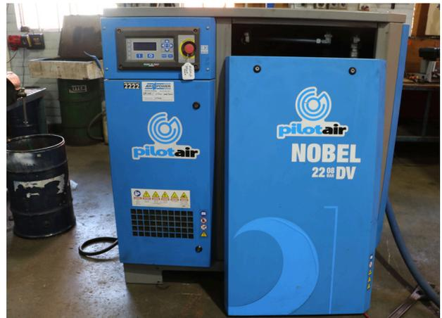
Full servicing of a Pilot Air Nobel compressor. Refurbished and tested before being deployed back to client's site.
