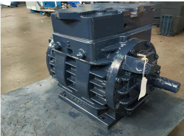
Full refurbishment of a Masport pump for **Abott's Liquid Salvage, Albany.** The pump's clearance was reset and exterior was spray painted. Pump was tested before being sent back to client.
